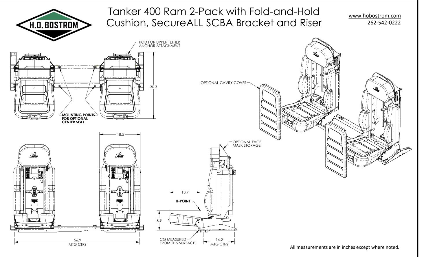
Seat dimensions are model-specific and subject to change; actual dimensions may vary slightly from the drawing. Contact H.O. Bostrom sales or customer service to identify specific seat features, possible applications, part numbers, and related dimensions. Designs and drawings are the property of H.O. Bostrom Company and are not to be reproduced or replicated. Copyright© 2023, H.O. Bostrom Company. All Rights Reserved.
