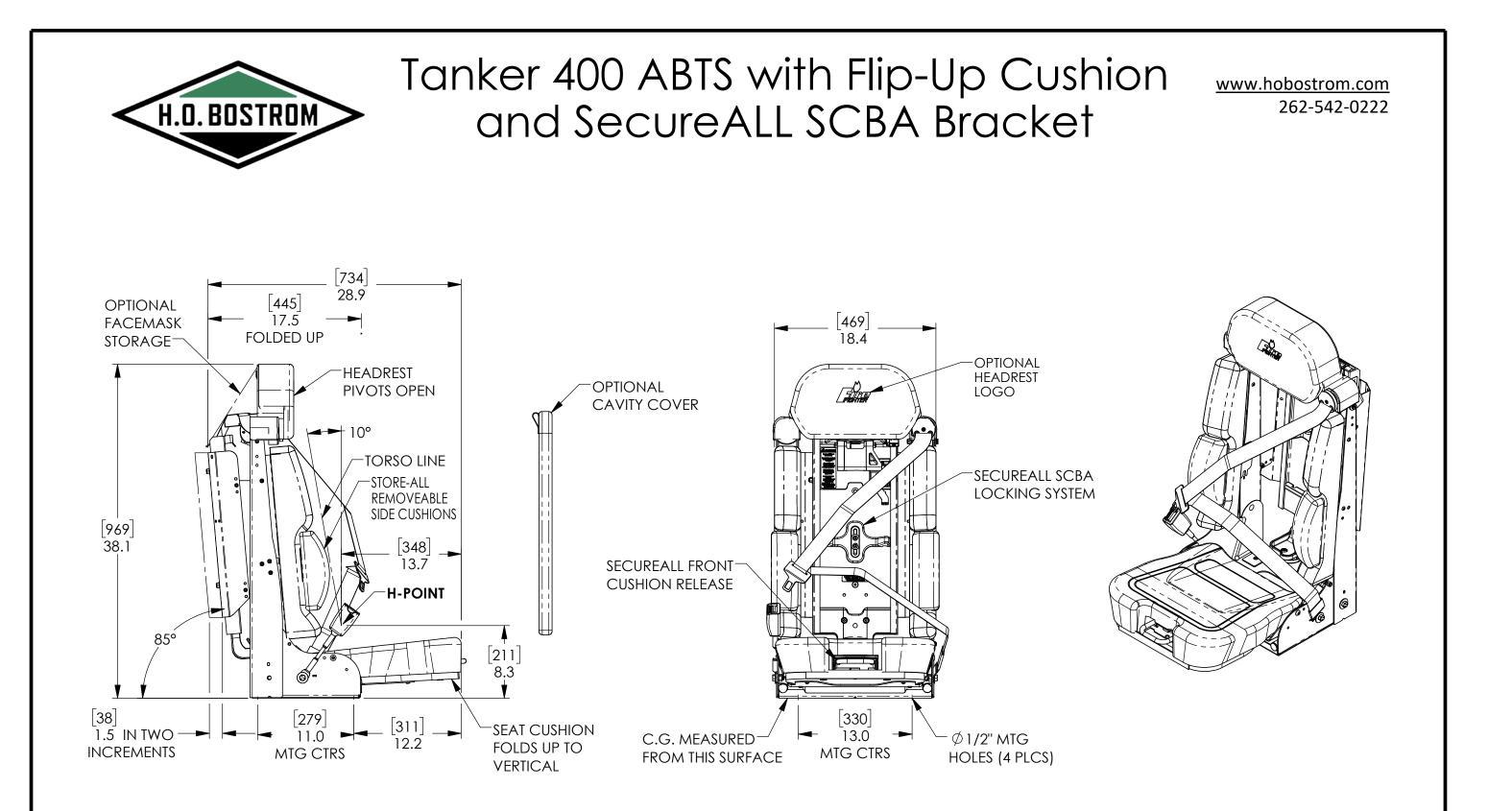
Seat dimensions are model-specific and subject to change; actual dimensions may vary slightly from the drawing. Contact H.O. Bostrom sales or customer service to identify specific seat features, possible applications, part numbers, and related dimensions. Designs and drawings are the property of H.O. Bostrom Company and are not to be reproduced or replicated. Copyright© 2023, H.O. Bostrom Company. All Rights Reserved.
