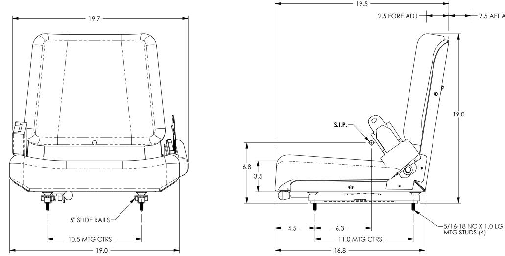
Seat dimensions are model-specific and subject to change; actual dimensions may vary slightly from the drawing. Contact H.O. Bostrom sales or customer service to identify specific seat features, possible applications, part numbers, and related dimensions. Designs and drawings are the property of H.O. Bostrom Company and are not to be reproduced or replicated. Copyright© 2023, H.O. Bostrom Company. All Rights Reserved.
